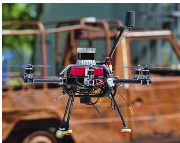
A research drone is used for three-dimensional measurement of the environment. The map can then be used to plan missions.
