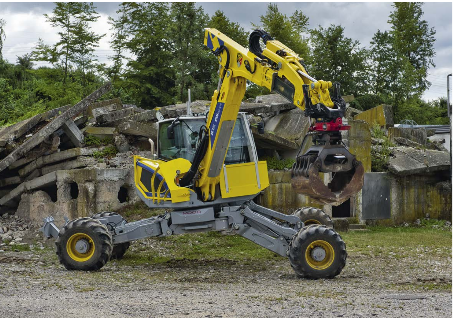
The largest four-legged robot at the SDRC has been equipped with a gripper, which enables objects weighing several tons to be moved.
