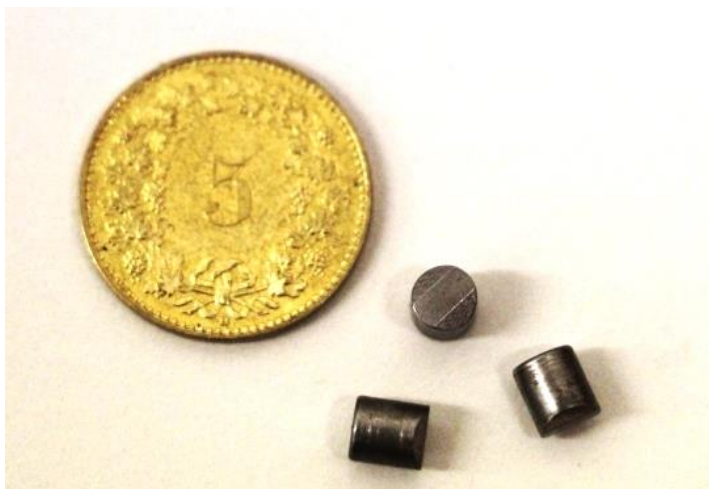
Figure 1: Fragment simulating projectiles FSP weighing 0.325g
