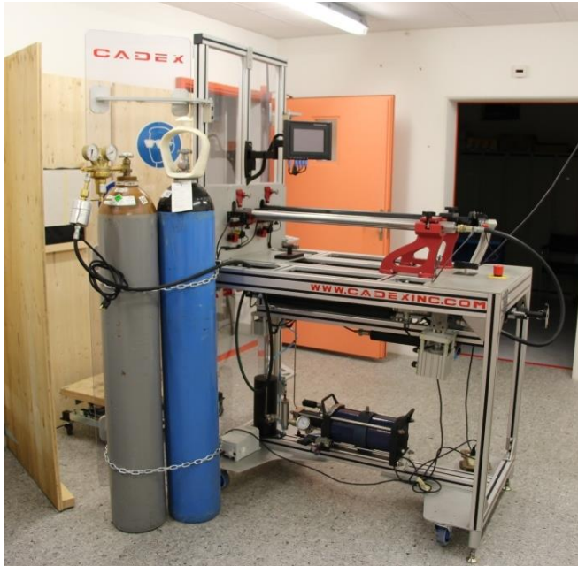
Figure 2: Test equipment for acceleration of minute fragments
