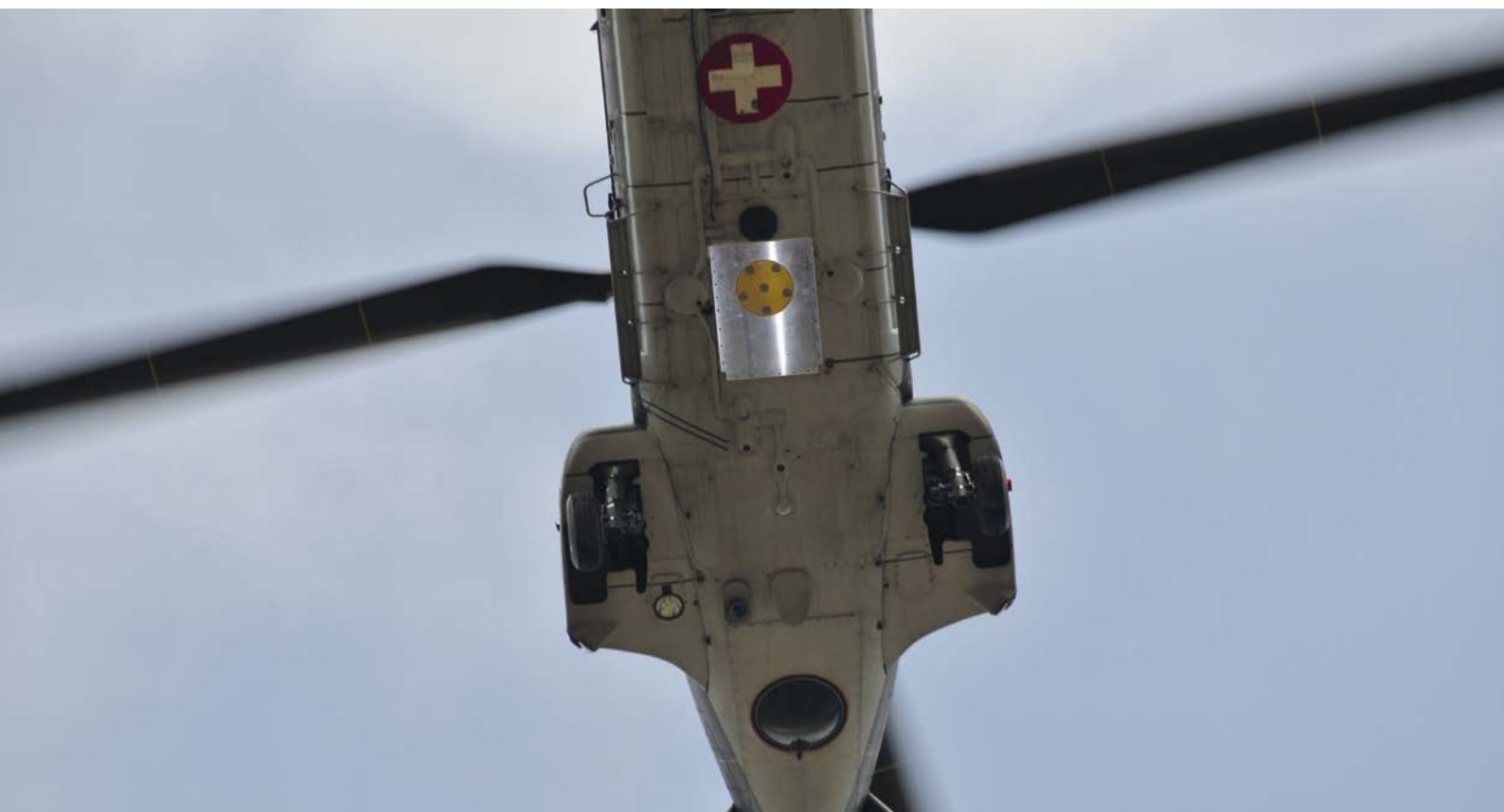
The technology demonstrator was attached to the underside of the helicopter.
