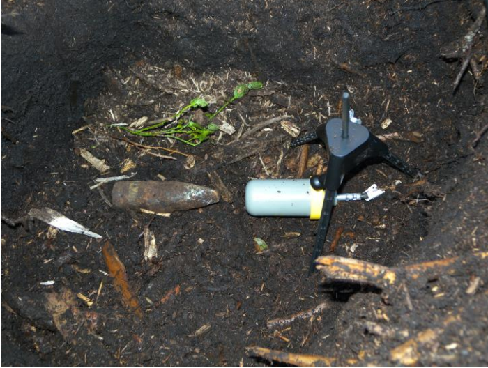
Fig. 2: Contactless destruction of blind (30 mm high-explosive aircraft cannon round)
