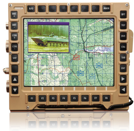
Abb2: The 10.4-inch SD7310 smart display from General Dynamics Canada is used in vetronics applications. Quelle: http://www.gd-ms.ca/
