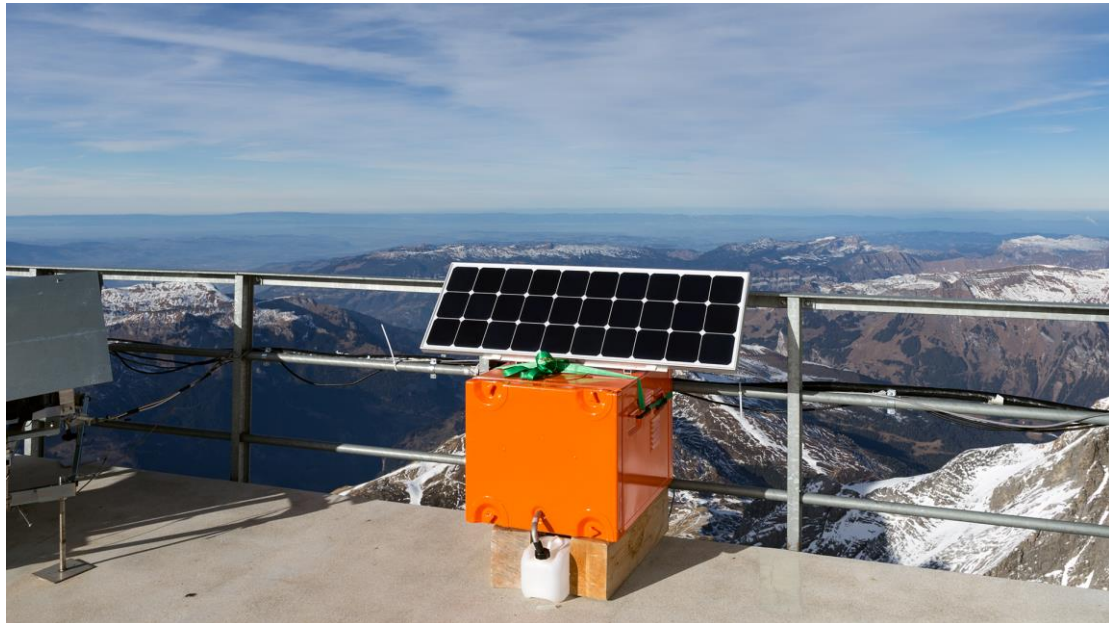
Figure 1. Methanol Fuel Cell in its weatherproof aluminium box with the attached auxiliary solar panel on the lower platform of the Sphinx observatory during the winter trials.
