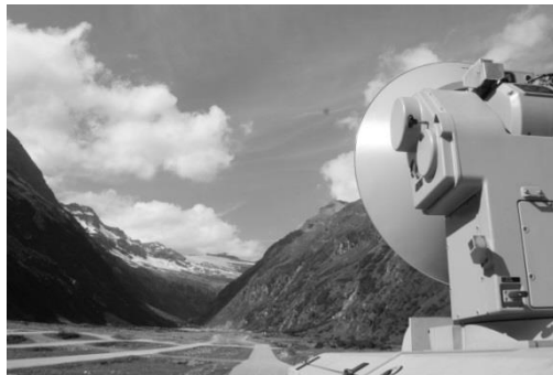
Figure 2 – "IRIS" trajectory tracking radar, Hinterrhein 2014
