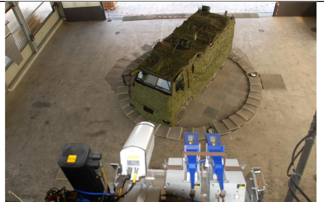
Radar antennae (in the foreground) measuring a rotating APC fitted with a camouflage kit
