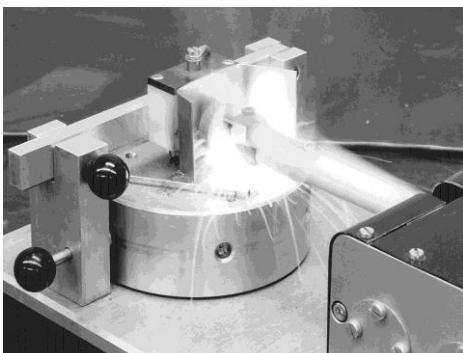
Measuring of electrostatic discharge in a round robin test to ascertain handling safety
