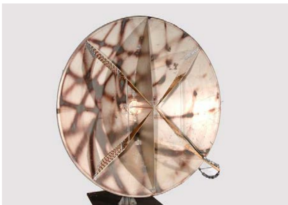
SWIRA (Swiss IRA): Ultra-wide-band antenna with frequency range 100 MHz - 4 GHz
