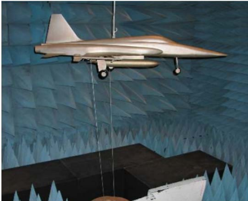
Model aircraft in the anechoic chamber
