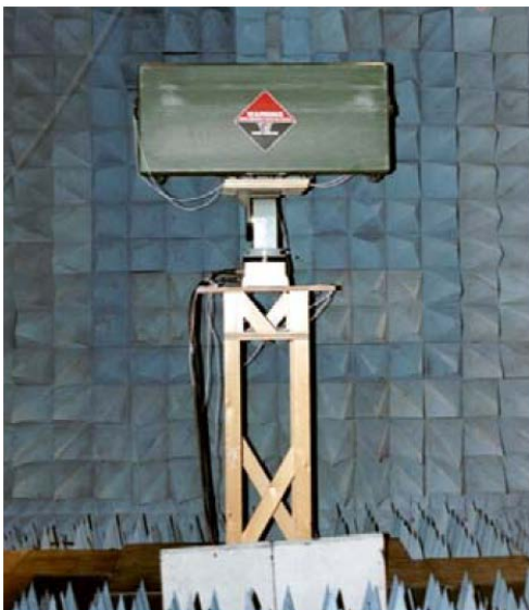
Measurement of antenna directional response patterns
