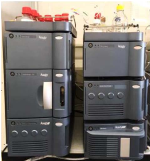
Ultra-high performance liquid chromatography (UHPLC) for analysing propellant powder at armasuisse S+T
